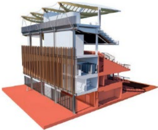
02 - New Steel Frame to the Upper Tier
